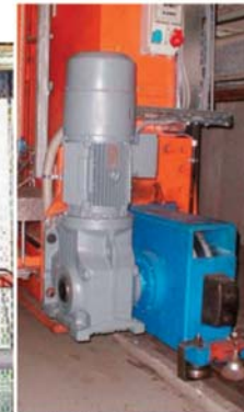
new carriage motor with gear
