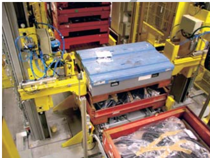
depalletting device with optical outline detection
