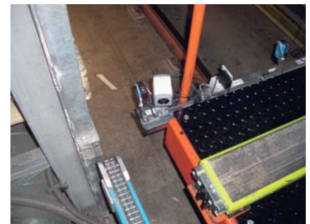
new telescopic fork with camera and new inspection sensor technology
